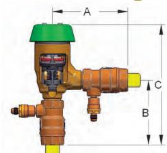
The Apollo' Model PVB 4A or PVBLF 4A Pressure Vacuum Breakers are designed to prevent contamination of potable water due to back-siphonage. An integral relief valve serves to reduce the possibility of damage due to intermittent freezing conditions. The modular check valve cartridge has a replaceable seat and a reversible silicone seat disc. Ball valves with stainless steel handles and nuts are standard.
