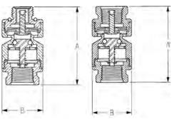
The Apollo® Series LFDUC is designed to provide protection against back-siphonage wherever a hose is connected to a faucet. The device consists of two independently acting checks with an intermediate relief port or vent. It is suitable for supply pressure up to 150 psig and a temperature range of 33°F-212°F. Not suitable for constant pressure conditions.
