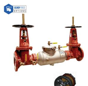
The Apollo® Model DCLF 4A Double Check Valves are designed to prevent contamination of the potable water supply due to back-siphonage or backpressure from substances that are objectionable, but non-health hazards. The TriForce™ center stem guided check valves feature replaceable and reversible silicone seat discs. The body is domestic stainless steel from 2-1/2"-8" and FDA epoxy coated ductile iron in the 10" and 12". Available with a wide variety of shutoff valve options.
