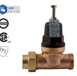
The Apollo® 36ELF is designed for residential and commercial applications to protect water supplies from excessive pressure. Excellent flow performance at low pressure drop. The dezincification resistant bronze body and dielectric polymer cage provide maximum corrosion resistance. Designed for easy in-line servicing with simple cartridge removal. They meet ASSE 1003 and CSA B356 standards. They are listed with IAPMO and the city of Los Angeles.
