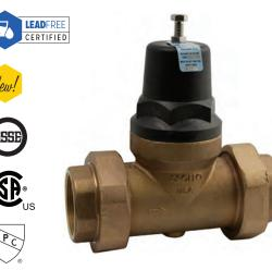
The new large diameter Apollo<sup>®</sup> 36ELF Lead Free Pressure Reducing Valve is designed to conserve water and protect water distribution systems by automatically reducing elevated supply pressures. The dezincification resistant bronze body, stainless steel adjusting screw and dielectric polymer cage provide maximum corrosion resistance. Designed for easy inline servicing with simple cartridge removal.
