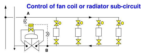
The differential pressure across the sub-circuit is maintained essentially constant irrespective of changes in flow-rate or mains pressure. This ensures that :
