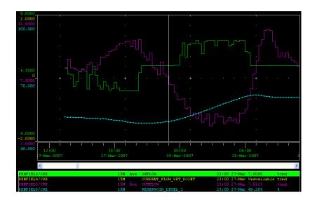
Before: The green line indicates poor flow control - moving erratically.
