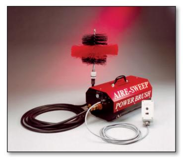
**REVERSIBILITY:** The cable system enables the operator to reverse the direction of the cable rotation, thereby reaching both sides of the ductwork. This results in faster and more efficient cleaning and excellent cable life. The specially designed bi-directional cable helps to prevent the cable breakage that is so common when standard cable systems are run in reverse.
