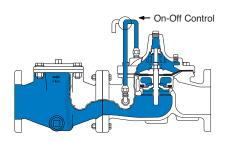
**Tight Closing Operation** When pressure from the valve inlet is applied to the cover chamber, the valve closes drip-tight.
