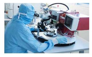
The entire production of the interdigital converters takes place in clean room conditions.
