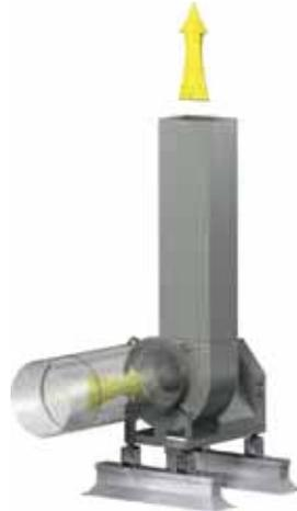
Typically used with remote fan mounting locations and ducting run along the roof deck. Slip fit or flanged connection to fan inlet. Recommended installation with three wheel diameters of straight duct prior to inlet to prevent airflow system effects.
