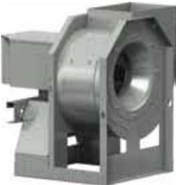
Available in belt or direct drive, arrangement 10 or 4, AMCA class 0, I or II. Options for spark resistance, high temperature or corrosive exhausts.
