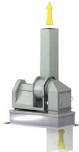
Positions the exhaust fan over the roof penetration. Compact installation minimizes roof deck space and leakage from multiple roof penetrations. Duct support provided to install duct drops in roof curb. Optional backdraft damper prevents airflow back into the building when fan is not in operation.
