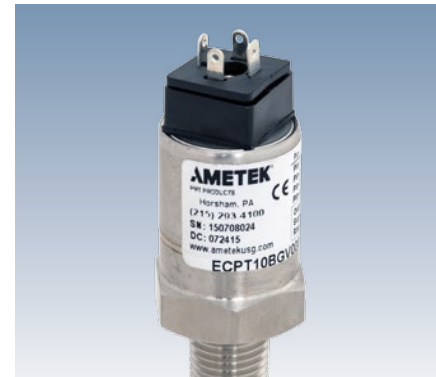
Model ECPT10 Low Cost Transducer: Pressure ranges: Vacuum to 0 psi through 0-10 000 psi • Accuracy: ± 1% full scale (BFSL) • Fatigue life: over 4 million cycles
