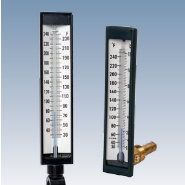
Model T-571 & T-572 Glass Tube Thermometers: 9" adjustable angle • 5½" low mount or low back mount connections • Dual temperature scales in °F & °C
