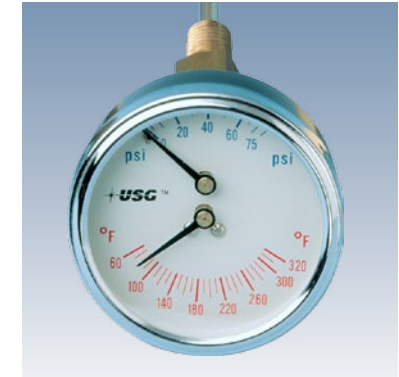
Model PT-1088 Boiler and Heater System Gauge: 2½" gauge size • Dial reads 0-75 psi/60-320° F • Short shank 0.78" or long shank 2.02"
