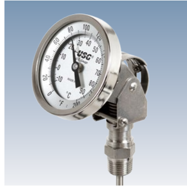
Model ADJ Adjustable Bi-metric Thermometer: 3" or 5" dial sizes • Standard stem lengths from 2½" through 12" • Custom stem lengths available
