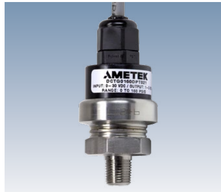
Model DCT Digital Transducer: Vacuum, compound, and gauge pressure ranges • Accuracy: ± 0.2% full scale (BFSL) • Outputs 4-20 mA, 1-5 VDC, 1-6 VDC, 0-5 VDC
