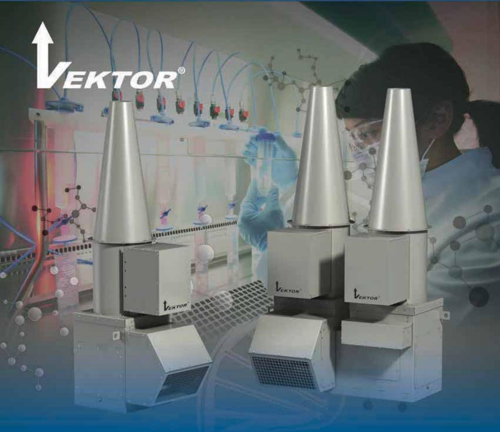
The Vektor®-H is a cost-effective, self-contained, high plume laboratory exhaust system designed to remove hazardous or noxious fumes from a laboratory, dilute the fumes with bypass air and expel them from the laboratory building so the fumes do not contaminate the roof area or are re-entrained into building make-up air systems.
