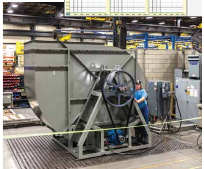
Assembled Fan Package on Vibration Test Stand
