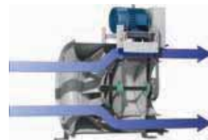
Mixed Flow QEI Fan: Slight airflow deflection from straight-through.
