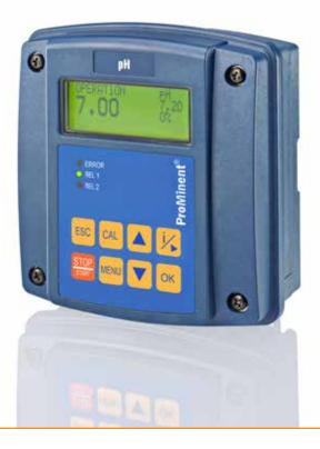
The **ProMinent® DULCOMETER® Compact** analyzer provides precise measurement and control of pH or ORP process variables. The pre-configured Compact can be programmed for either pH or ORP control without having to purchase a separate analyzer. Temperature compensation for pH can be added using an optional PT 1000 sensor. The Compact comes standard with pulse relay for pump control, configurable analog output and configurable power relay.
