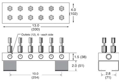
Weight: 13 lbs (5,9 kgs) Orifice Size: 0.19" Weight: 24 lbs (10,9 kgs) Orifice Size: 0.19"
