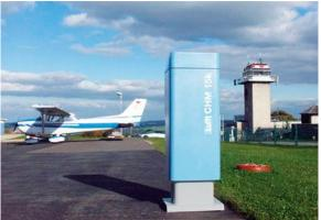
One important use of the ceilometer is to determine cloud ceilings at airports. CHM 8k can identify up to 9 cloud layers and is very sensitive even at ground level
