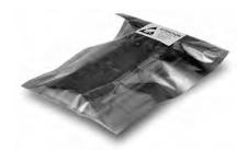
This static shield bag offers total ESD protection, whether you're transporting ESD-susceptible products across the room or across the country. The outer layer of the bag consists of an abrasion-resistant polyester, while the antistatic polyethylene inner layer retards triboelectric static charging from inside the bag.
