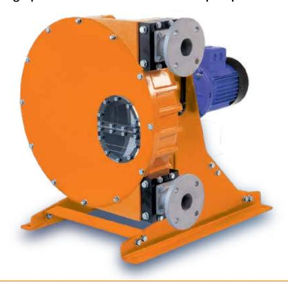
The **DulcoFlex DFD** is a hose pump designed for pressures up to **232 psi** and flow rates up to **160 gpm**. The unique shoe design is made of steel for smoother and cooler compression. The DFD uses safe **DulcoLube** oil for the shoe lubrication. With suction lifts up to **29 feet**, the DulcoFlex DFD is a great choice for difficult pumping applications.
