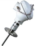
RTD assembly with FDA Approved Poly Connection Head                            | Yes                | Tri-Clamp          | Yes | 4-20 mA, 0-5 VDC, HART | Various from -50 to 400) Custom Ranges Available | ±(0.2°F + 0.10% of calibrated span) with two-point calibration | IP65             |
