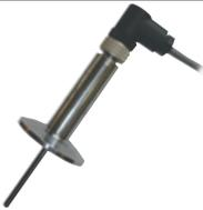
RTD with Integrated Transmitter                                                 | Yes                | Tri-Clamp®         | Yes | 4-20 mA                | Various from -60 to 320 Custom Ranges Available  | ±(0.2°F + 0.10% of calibrated span) with two-point calibration | IP67/<br>NEMA 6  |
