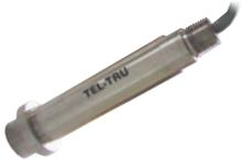
Homogenizer Pressure Transmitter Models P341 | N/A                | Standard Gaulin Homogenizer                                                           | N/A | 4-20 mA, 0-5 VDC, 1-2 mV/V | 0/100 up to 0/20,000 psi  | ±0.5% FSO  | NEMA 4X          |
