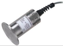
Sanitary Pressure Transmitter Model P321     | Yes                | Tri-Clamp or Cherry-Burrell                                                           | Yes | 4-20 mA, 0-5 VDC           | 0/3 up to 0/1,000 psi     | ±0.25% FSO | NEMA 4X          |
