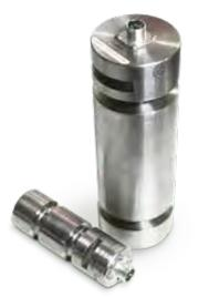
A key component for MSI's integrated overhead weighing solutions is the Load Pin Sensor. Typically designed and manufactured specifically to each integrated solution, the MSI load pin is strictly industrial grade. Each load pin design is precision machined from 17-4 stainless steel for safety, strength and corrosion resistance.
