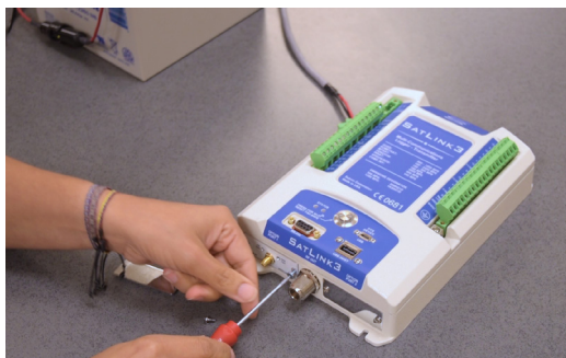
Cellular Card Installation
