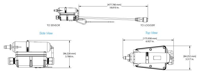
Desiccant Hub Assemblies for use with portable FL900 Series Loggers and Marsh-McBirney Flo-Logger. (Sensor cable for use with FLO-STATION will not contain a desiccant hub and will have bare wires on cable end.)
