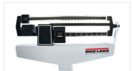
Weigh beam with lb markings
