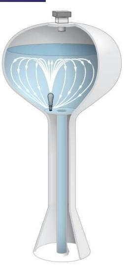
Active mixing and ventilation are the first steps in THM removal. The PAX Mixer continually introduces THM-concentrated water to the surface where THMs are volatilized and evacuated by the PAX Coaxial Powervent<sup>®</sup>.
