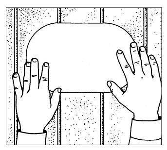
**SELF-ADHESIVE TEMPLATES** are also provided so that the duct opening can be cut without expensive lay-out.
