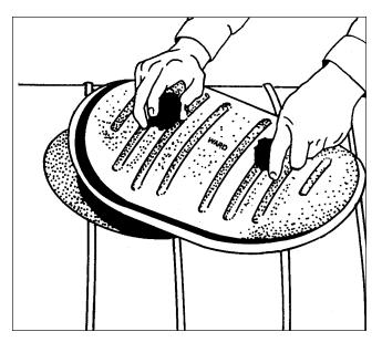
**EASY INSTALLATION** after door opening has been cut, unscrew handles or door in insert in the opening, align then tighten knobs.
