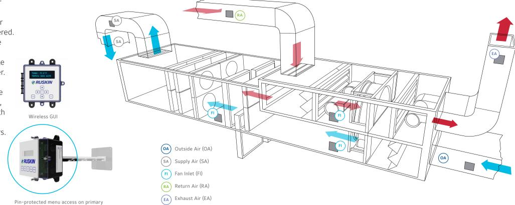
Every air measurement station has a primary. It can be located on the end of the probe, as shown above or as a separate box remotely located up to 500 feet away from the air measurement station. The primary displays airflow and temperature during normal operation and allows easy menu access without removing covers or screws. The Remote Graphic User Interface (GUI) provides the same display and menus, wired or wirelessly.
