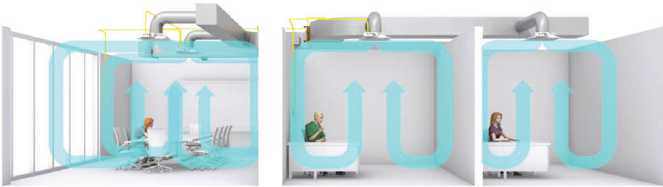
Each Thermo-Fuser VAV diffuser has a built in thermostat.
