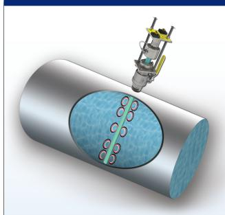
The FPI Mag operates based on Faraday's Law of Electromagnetic Induction: When water (a conductor) moves through a magnetic field, it produces a voltage that is directly proportional to the velocity of the conductor.
