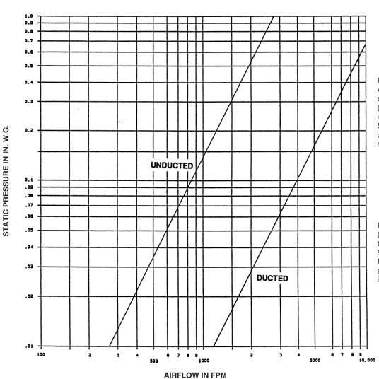
Performance curves based on AMCA Standard 500 using test setup apparatus figure 5.3 (damper installed with duct upstream and downstream). Static pressure and CFM are corrected to .075 lb/cu ft air density.
