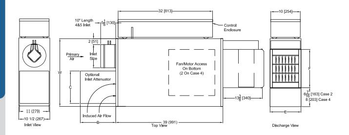
The standard location for control enclosure is Left Hand on Model FCL. Looking in the direction of airflow, the control enclosure is on the left.
