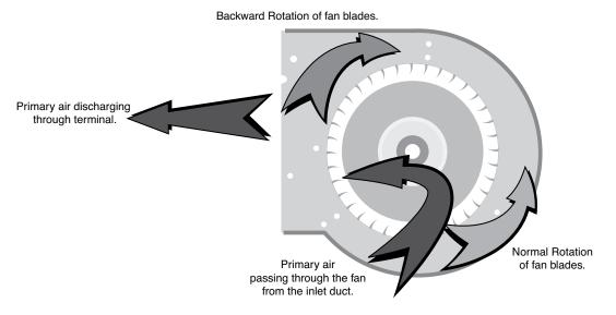
Constant fan boxes must have means to coordinate energizing the fan motor with start up of the Primary Fan System to prevent the reverse rotation or a positive method to create enough motor torque to reverse the rotation of the fan wheel.
