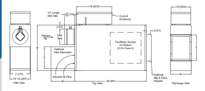
The standard location for control enclosure is Left Hand on Model FCL. Looking in the direction of airflow, the control enclosure is on the left.
