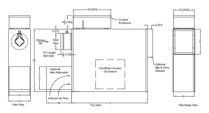
The standard location for control enclosure is Left Hand on Model FVL. Looking in the direction of airflow, the control enclosure is on the left.
