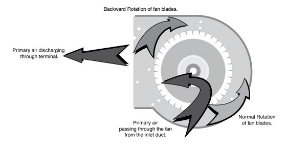
Systems with constant fan boxes must have a means to coordinate energizing the fan motor with start up of the Primary Fan System to prevent the reverse rotation of the terminal unit family. This is accomplished by proper operation and staging by the building control system. Another option is to create enough motor torque to reverse the rotation of the fan wheel.
