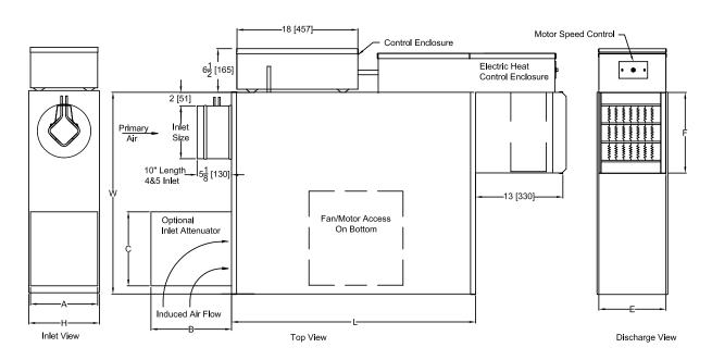
The standard location for control enclosure is Left Hand on Model FVL. Looking in the direction of airflow, the control enclosure is on the left.
