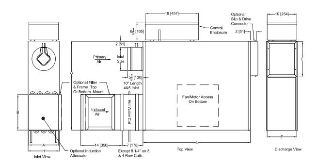
The standard location for control enclosure is Left Hand on Model FVL. Looking in the direction of airflow, the control enclosure is on the left.
