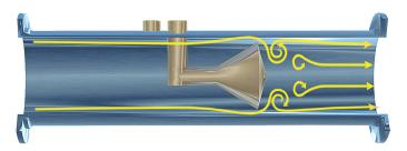
The contour-shaped cone directs the flow away from the cone, keeping the beta edge free from wear. Therefore, V-cone flow meters rarely require recalibration or replacement.
