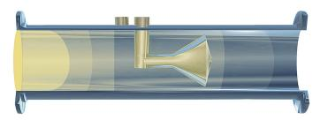
As the flow approaches the cone, the flow profile "flattens" toward the shape of a well developed profile—even in extreme flow conditions.
