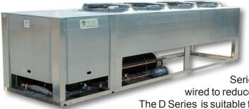
Century Refrigeration's D Series air cooled condensing units are specifically designed to meet the demands of multiple load applications required for commercial and industrial duty refrigeration applications. D Series units are vertical air discharge condensing units that utilize a horizontal condenser coil, high volume condenser fans, and a separate subcooling circuit in the condenser to maximize performance. Our D Series condensing units arrive at the job site pre-piped and pre-
