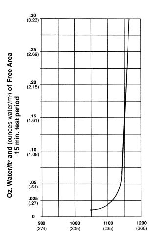
Free Area Velocity in feet and (meters) per minute Standard air .075 lb/ft³
