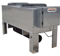
Technical Systems Series 10 air cooled condensers can be rated for all refrigerants, including R22, 407c, 134a, and 410a. Fan type and performance can be configured to meet your unique sound requirements for the ultimate acoustical solution. Unlike typical products with microchannel or "enhanced" fins coils, Series 10 plate-fin coils remain fully cleanable with simple corrugated fins. This means reliability over time and reduced maintenance costs.
