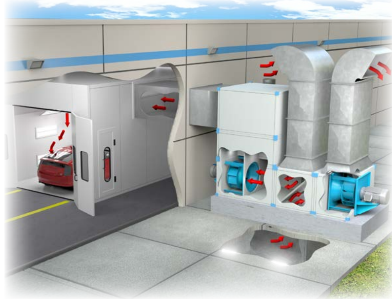
Paint Booth Ventilation
