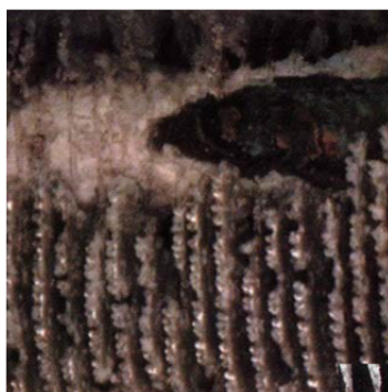
Untreated coils after 4,000 hours in salt spray chamber.
