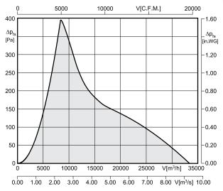
NOTE: The above air performance curves have been established according to DIN EN ISO 5801.
