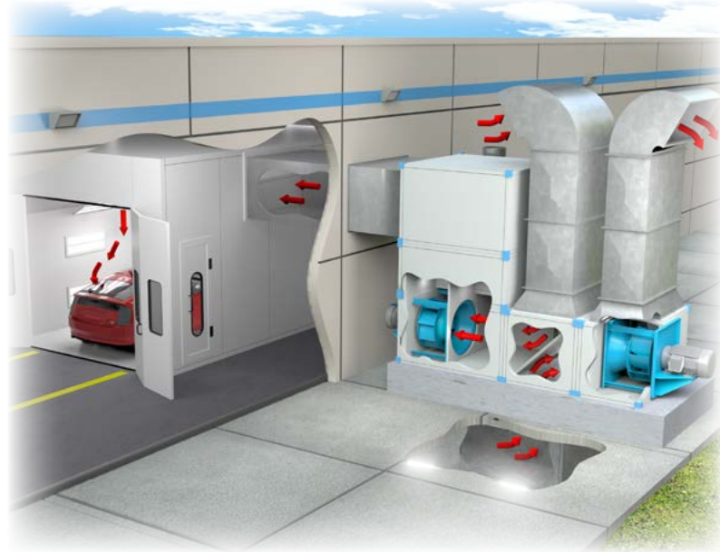
Paint Booth Ventilation
