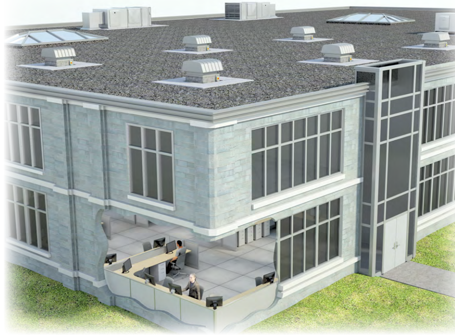
General HVAC Exhaust (Hooded Roof Exhausters)
