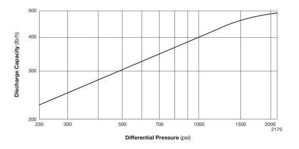
1. Differential pressure is the difference between the inlet and outlet pressure of the trap. 2. Recommended safety factor: at least 2.
