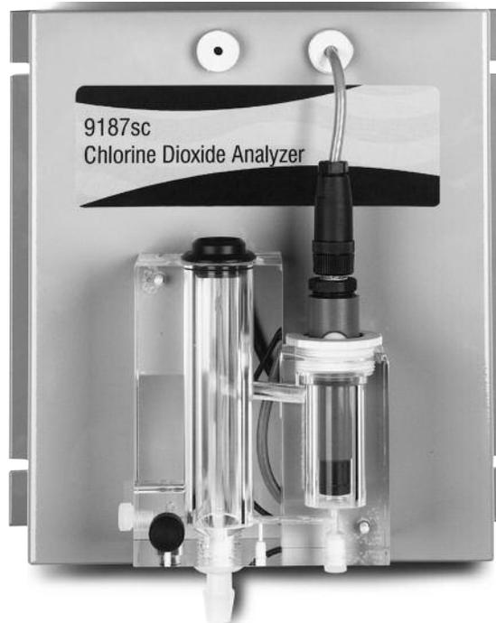
*Selective membrane used in the Hach 9187 sc Amperometric Chlorine Dioxide Sensor avoids interferences from chlorine for accurate, low level measurements. Electrode membranes are pre-mounted for easy replacement.*
