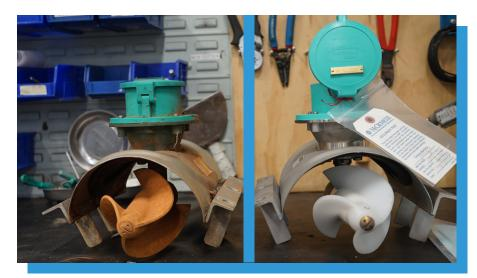
**Left:** a saddle-style Water Specialties propeller meter ready to undergo a complete meter repair.
