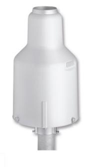
The OTT Pluvio<sup>2</sup> L is an all-weather precipitation gauge that uses superior weight-based technology to measure the amount and intensity of rain, snow, and hail. Developed in conjunction with industry-leading meteorological services, the OTT Pluvio<sup>2</sup> L employs a high-precision load cell and algorithms that compensate for wind, temperature, and evaporation, ensuring the highest accuracy precipitation measurements over time.
