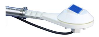
WET The ADCON Leaf Wetness Sensor was developed to provide users with a robust and low-maintenance alternative to the traditional style sensors using sheets of paper or human or animal hair. A grid of conductive tracks, etched onto a Teflon-coated ceramic plate reliably simulates the surface of a leaf and outputs a range of readings between 0 and 10.
