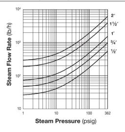
The chart above is used to determine the steam flow rate through the DC7 separator. It is based on a steam velocity of 100 ft/s. For other velocities, calculate the flow rate as follows:
