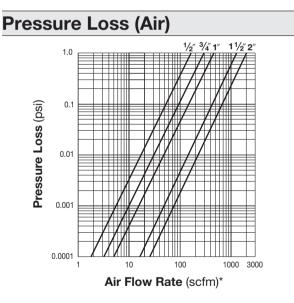
The pressure loss chart is based on an air pressure of 150 psig. For other pressures, multiply the air flow rate by the correction factor given in the table below. Use the result on the pressure loss chart.
