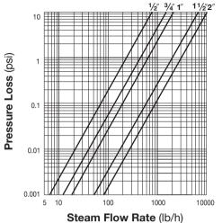
The pressure loss chart is based on a steam pressure of 150 psig. For other pressures, multiply the steam flow rate by the correction factor given in the table below. Use the result on the pressure loss chart.
