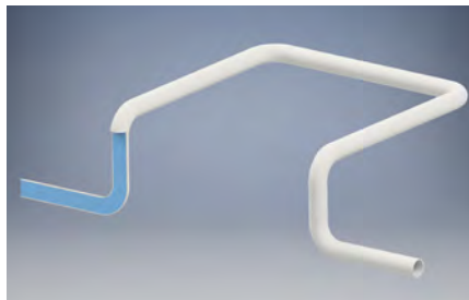
FIG. 17. Piping designers sometimes incorrectly believe that condensate return lines contain only water flow.
