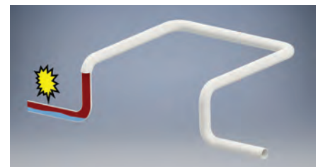
FIG. 19. Danger: Vertical loops on CR cannot drain condensate, and the level can build with no way to move upward.
