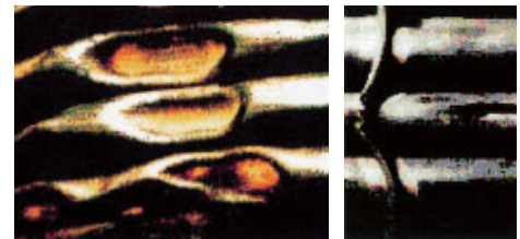
Water hammer damage to tubes and stays
