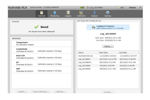
The Hydrolab Operating Software is the PC-based application for interfacing with Hydrolab HL Series sondes, the Hydrolab Surveyor HL, and Hydrolab communications modules. It is designed for intuitive water quality data collection, sensor calibration, settings adjustment, and metadata access
